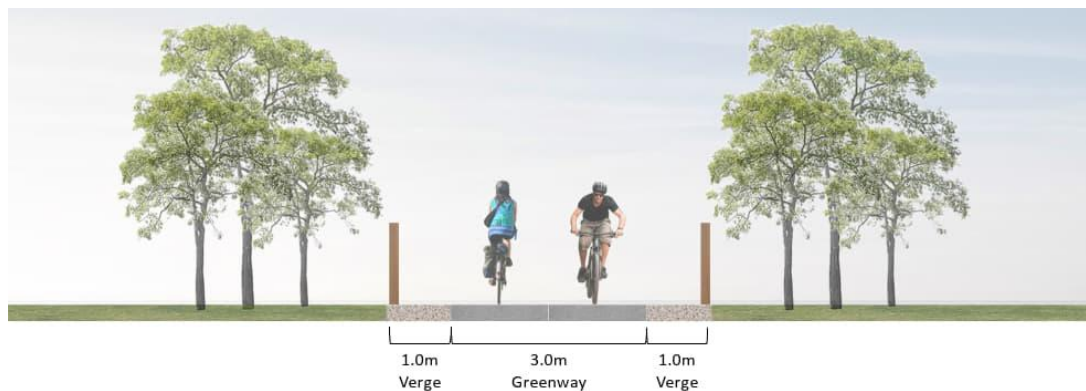
Figure 4-13 - Typical Cross Section of 3.00m Wide Greenway
