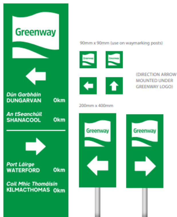
Figure 4-40 - On route directional signage
